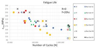
The fatigue resistance is characterized by a high scatter of results: two distinct behaviour are observed among samples manufactured in X, Y directions, under three different combination of laser power, exposure time, hatch distance and point distance
