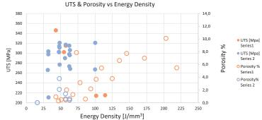
The material tensile strength is correlated to microstructure morphology:
