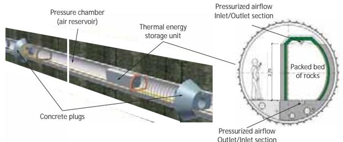
Fig. 2: AA-CAES pilot plant layout (l.h.s.) and tunnel cross-section (r.h.s.). Courtesy of ALACAES SA.
