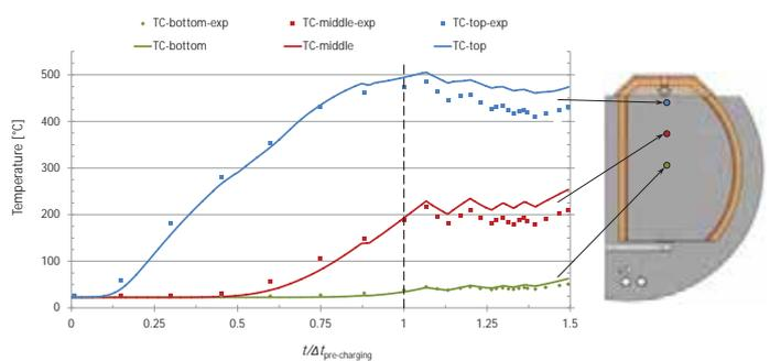
Fig. 3: Comparison between CFD simulation results (solid lines) and experimental data (markers).
