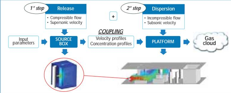
**In a nutshell:** The accidental phenomenon (highly pressurised gas release) is split in two phases → **supersonic release and dispersion**.
